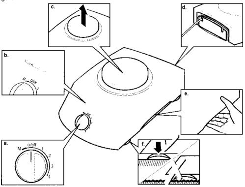
no flour or oil on the surface. A clean smooth surface will provide the best footing for the suction cup feet on the power unit and will limit slipping and/or "walking."
